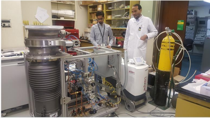
Engineers are testing the new vacuum system with leak detector before installation
