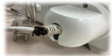
(Figure 1): Over-stretching and cut on the tip of the power cable.
