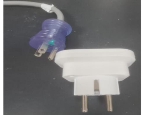
Figure 2 Power Cable of US-110V type with Power Adapter with Schuko-220V fitted pins
